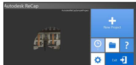
Begin by selecting scan files to import, and then use the tools inside of Autodesk ReCap to work with the scanned data. Use the Home tile menu to save the current project as a Point Cloud Project file (RCP) or export to a Point cloud Scan file (RCS). Both can be used in AutoCAD.
