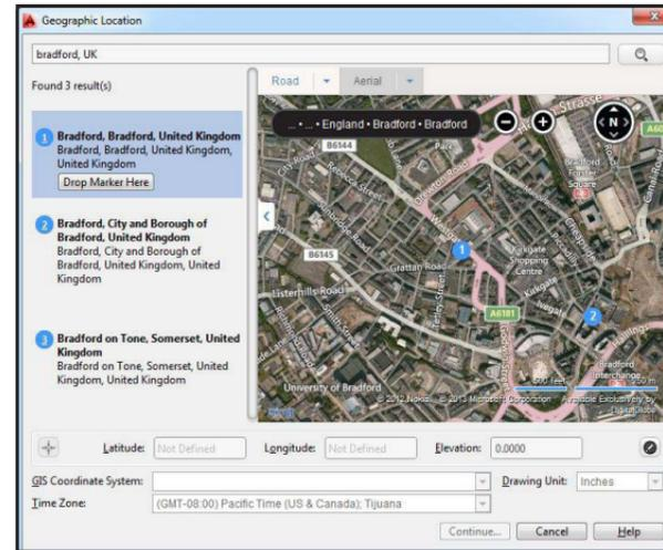
Set a geographic location using the Set Location tool (Insert tab). Easily search for an address or latitude and longitude from a map (if signed into your Autodesk account) or by selecting a KML/KMZ file.
