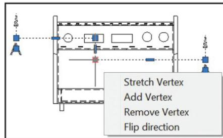
Grips on the section view, hatches and section view label allow you to make a variety of modifications.
