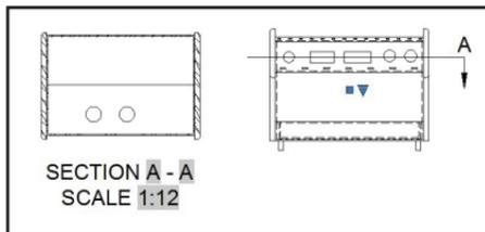
Use the Edit Components tool to modify the objects used in the Section View. If a component is set to none, it will not be sectioned.
