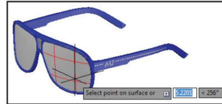
You can change the direction of the isolines, select a chain or draw a spline on the curved surface.
